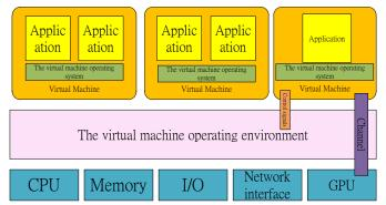
Figure 3 Architecture of GPU Virtualization
